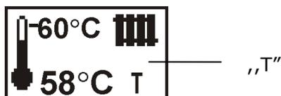
Drawing 34 View of the main window after activation of thermostat
