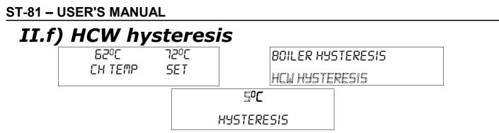
This option can be used to set the value of the hysteresis of the boiler set temperature. It is the difference between the set temperature (that is the boiler required temperature) and the actual boiler temperature (e.g. if the set temperature has the value of 55°C, and the hysteresis is 5°C. After the set temperature (55°C) is reached the HCW pump will switch off and the CH pump will switch on. The HCW pump will restart if the temperature decreases to 50°C.
