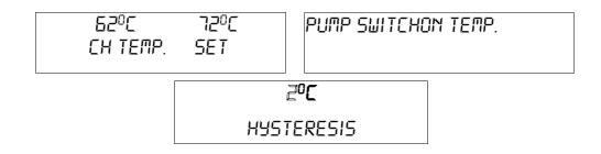
This option can be used to set the hysteresis of the set temperature. It is the difference between the temperature of start of the suspension mode and the temperature of restarting the operation mode (e.g. when value of the set temperature is 60°C and hysteresis is 2°C, the start of the suspension mode will take place at 60°C, whereas the restart of the operation mode will take place at 58°C. Hysteresis can be set in the range between 2°C and 6°C.
