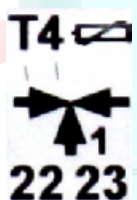
Fig.24. Identification of mixing valve temperature sensor connecting terminals.
