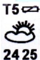
Fig.25. Identification of weather sensor connecting terminals .
